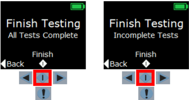
Figure 49: Clinic Base Station Finish Testing Screen. All tests complete (left); tests remaining (right).
